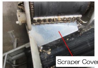
Preventing scraped manure going under the conveyor belt
