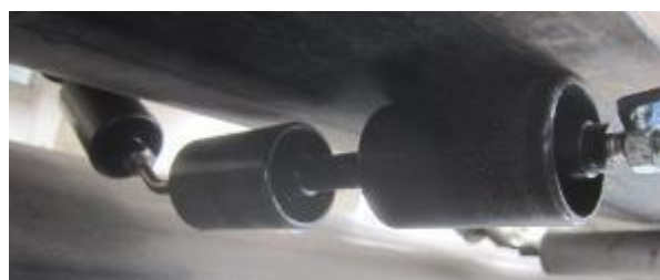
Nylon "Carrier" Roller to minimize manure sticking.
