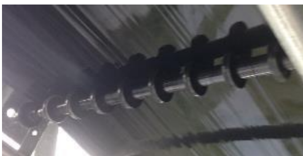
Nylon separated "Return" Roller to minimize manure sticking.
