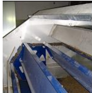
Reverse unit delivering manure to the lower tier
