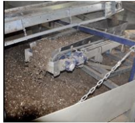
Spreader evenly filling manure on the plate
