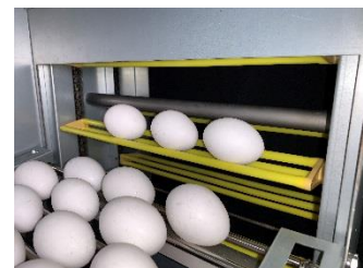
2 Air-cushion Gentle Bar Receives eggs softly with an air-cushioning effect.
