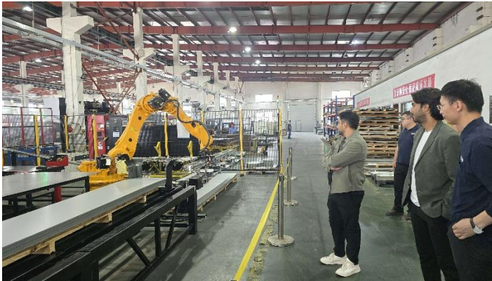
Sheet metal processing by Robot
